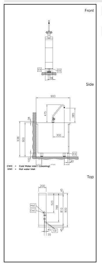
Inlet water line size: 3/4" Incoming Cold/hot Water line 3/4"
